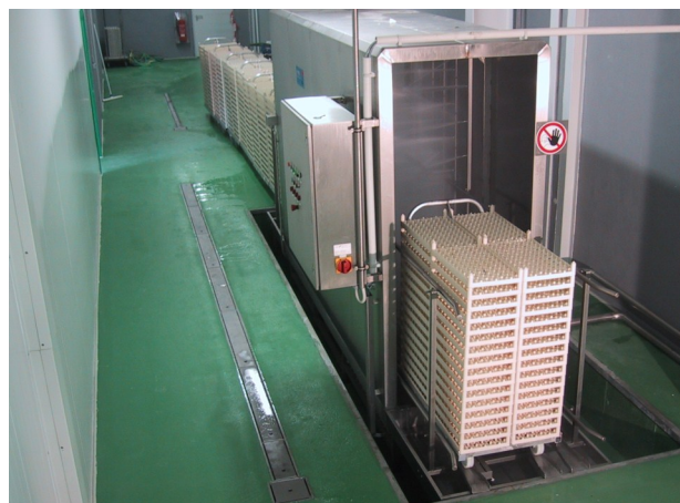
Washing machine Mafo 340MLPH with separate tank unit for extra low infeed
