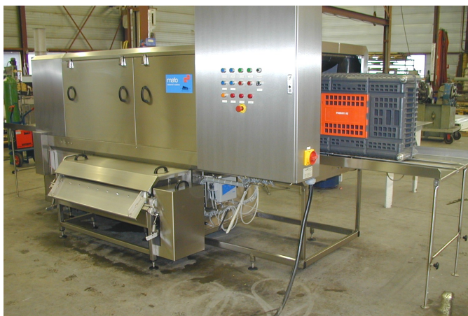
washing machine Mafo 340MPV For live bird crates.
