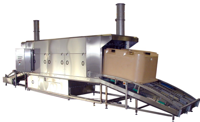
Washing machine 450MBH For pallet boxes.
