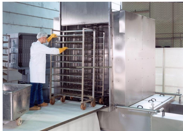
Cabin washing machine Mafo 250K For smoke racks .
